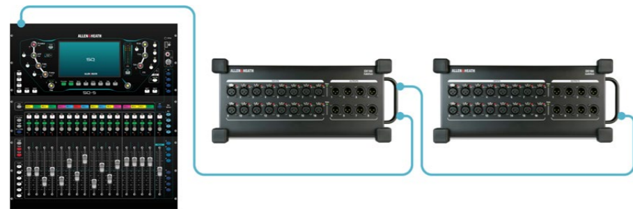
SQ + 2 x DX168 32 remote inputs + 16 remote outputs
