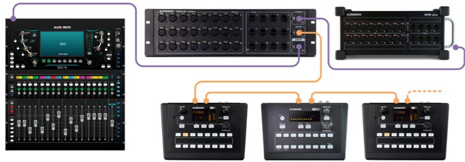
SQ + AR2412 + AB168 + ME system 40 remote inputs + 20 remote outputs + ME system
